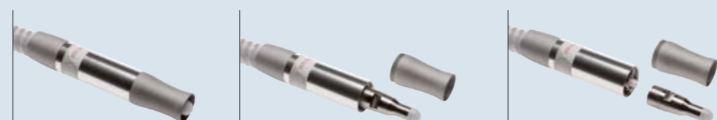
1. Unscrew the handpiece cover 2. Unscrew collet chuck 3. Screw the new collets chuck, screw the cover. Ready!
